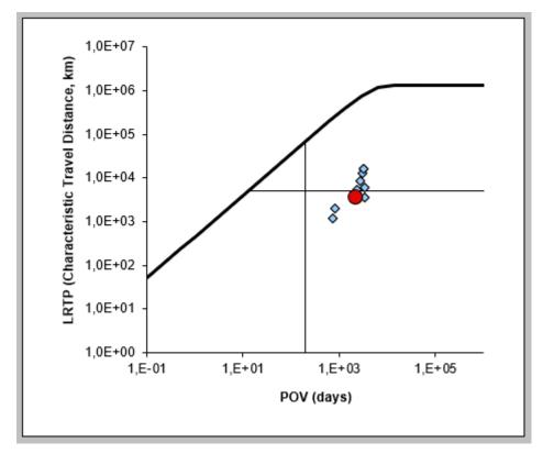
Figure 2: Graphical output for CTD of melamine assuming substance being "not biodegradable"; output in comparison to 'Generic PCB homologues'.
