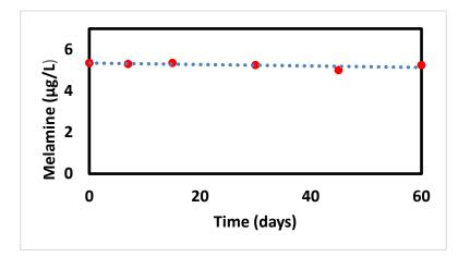
Figure 1: Concentration of melamine ( $\mu$ g/L) in a surface water test system in course of time (days). Data were shown as mean value of two individual bottles for each sampling point. Please note: Error bars indicating standard deviation are included in this figure. However, as the standard deviation resulted in values up to 0.071  $\mu$ g/L only, the error bars are hardly noticeable in the plot.
