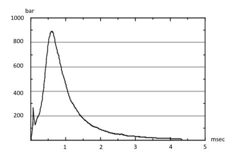
Figure E-5. Progress of chamber pressure during the firing of a shot.
