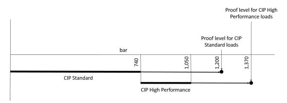
Figure E-6. Chamber pressure and proof limits according to CIP regulations<sup>118</sup>.
