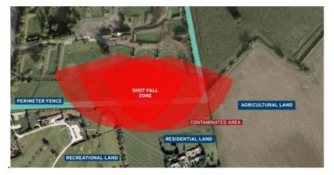
Figure 1-17: Example of lead shot deposition from a shotgun range on lands with different zoning (Victorian EPA, 2019)
