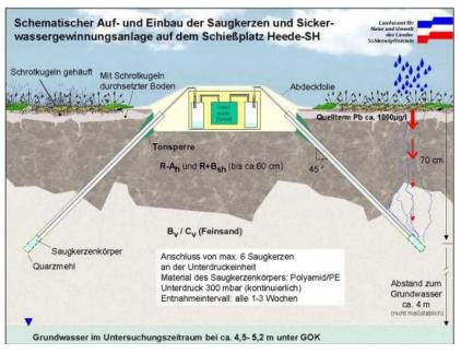
Figure 1-12: Example for measurement of seepage water in a shooting range (Schleswig-Holstein LANU, 2005)
