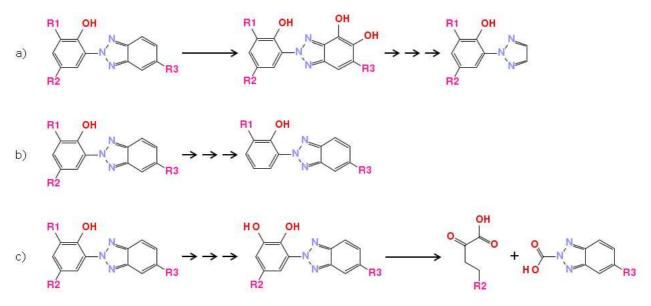
Figure 1: Proposed simplified mechanisms for the degradation of the phenolic benzotriazoles. a) Degradation of the benzotriazole moiety; b) Degradation of side chain R2; c) Degradation of side chain R1 leading to the ringcleavage of the phenolic ring R1, R2: alkyl; R3: H or Cl. Side reactions are for the sake of simplicity not considered here.
