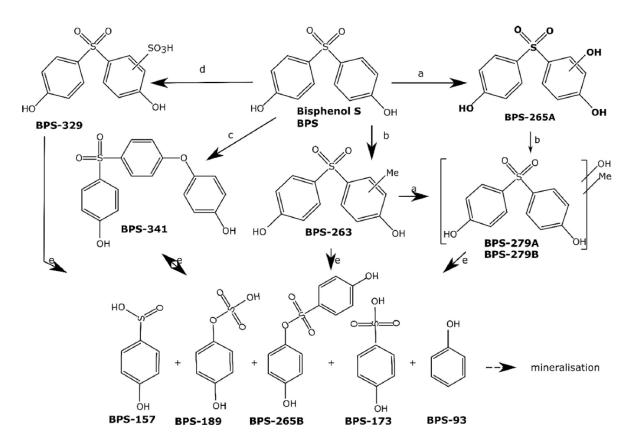
**Figure 1: proposed biodegradation pathway of BPS in activated sludge** (a: hydroxylation, b: methylation, c: the coupling of smaller BPS moieties, d: sulphonation and e: cleavage of the S–C bond, dashed arrows; not identified) (from Kovačič *et al.*, 2021).
