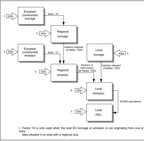
Figure 3.2.2 Flowchart for calculating the (PE)C, the entry for the calculations is depending on the submitted information.
