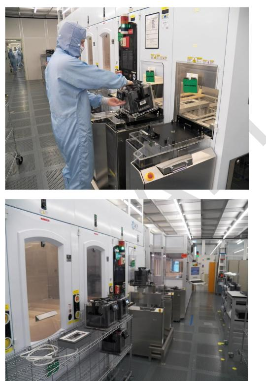
NMP for semiconductor use in wafer cleaning and as a solvent process is performed inside a closed manufacturing equipment system which is itself inside a controlled environment known as a 'clean room'. There is no contact between the workers and NMP during the normal semiconductor manufacturing processing and during this loading/unloading process of the wafers in batch.
