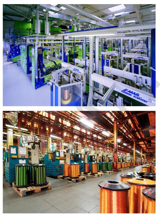
*Figure X01.1:* Two pictures of enameling machines in a wire coating factory.
