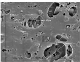
Figure 1: Detailed view of the micropores of a breathable backsheet (Counts et al., 2014)
