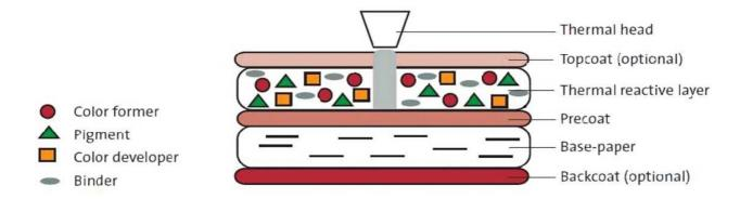
As illustrated in the Figure 3 above, the thermal paper is basically composed of a base paper all over which a thermo-coating is applied in a coating machine. This thermo-coating contains the principal functional components and forms the thermal reactive layer of the thermal paper. This layer is made up of 4 components:
