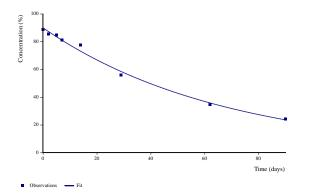
Figure 4. Fitted SFO curve for degradation in sandy clay loam (Dzialo 1988)
