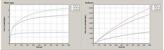
As the PEC:PNEC ratio including the regional background concentration is 0.991 after 500 days, an exceeding of the PNEC is likely during the service life of the sheet piling due to accumulation of copper in sediments. Consequently, unacceptable risks for the aquatic environment are expected due to accumulation of copper in sediments when preserved wood is applied large scale in water (e.g. sheet pilings).
