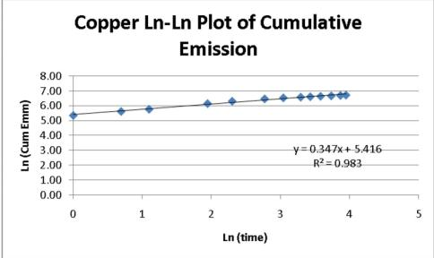
Figure B7. 1.2-6: Log-Log Plot of the Copper Cumulative Emission data
