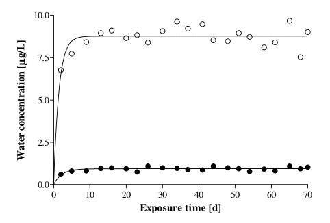
**Figure 1:** Water concentrations in a flow-through study with musk xylene at nominal concentrations of 1 ( $\bullet$ ) and 10 ( $\circ$ ) µg/l.
